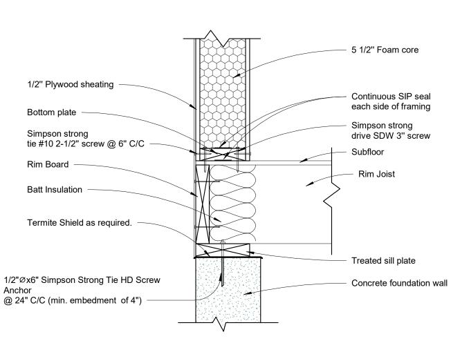
ALL SIP JOINTS SHALL BE AIR SEALED WITH SIP SEAL AND/OR SIP SEAL VAPOR TAPE. FOLLOW SIP MANUFACTURER'S RECOMMENDATIONS FOR SIP TAPE WIDTHS AND SEALANT PATTERN AND THICKNESSES
