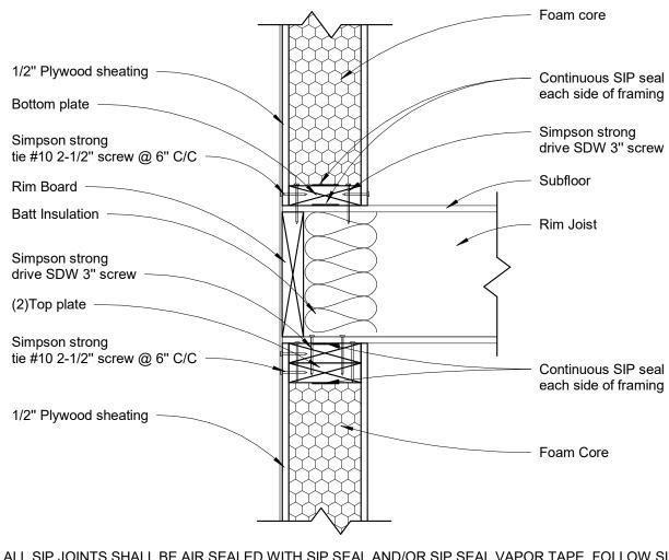
ALL SIP JOINTS SHALL BE AIR SEALED WITH SIP SEAL AND/OR SIP SEAL VAPOR TAPE. FOLLOW SIP MANUFACTURER'S RECOMMENDATIONS FOR SIP TAPE WIDTHS AND SEALANT PATTERN AND THICKNESSES
